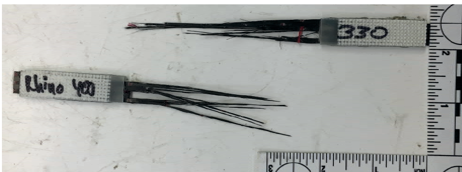
Figure 1.3 – Representative SGM failure mode, where 'S' is for longitudinal splitting; 'G' is at the gauge and 'M' middle. Scale in inches.
